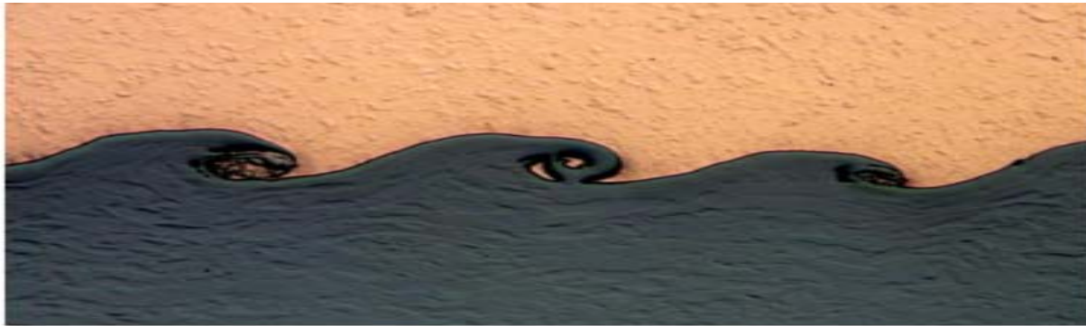
Figure 2. Typical explosion weld bondline. Note wavy fluid-like behavior.
