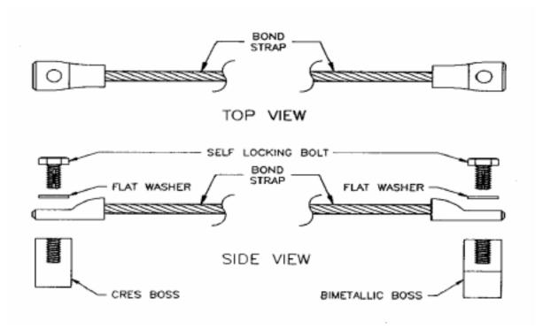
FIGURE 1. Type I bond strap assembly and associated components.
