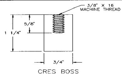
1. Bolt holes shall not penetrate through bondlines of bimetallic transition layer.
