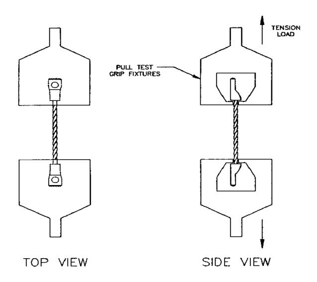
1. Grips shall be designed to transfer load uniformly to the base of lugs, across the diameter of lug.
